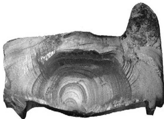
Figure 1. Fracture surface of the broken train wheel [1].
