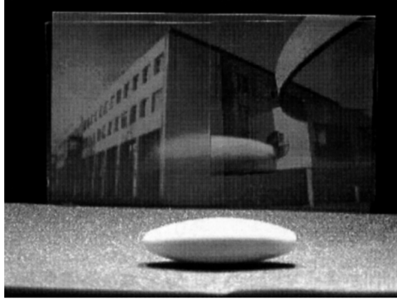
Figure 4 Difference in images formed of a white object. Left side is coated with AS-AG plastic, and the right side is uncoated. The coated side shows significantly reduced reflection. Image obtained from ref.[12] with permission from Elsevier.
