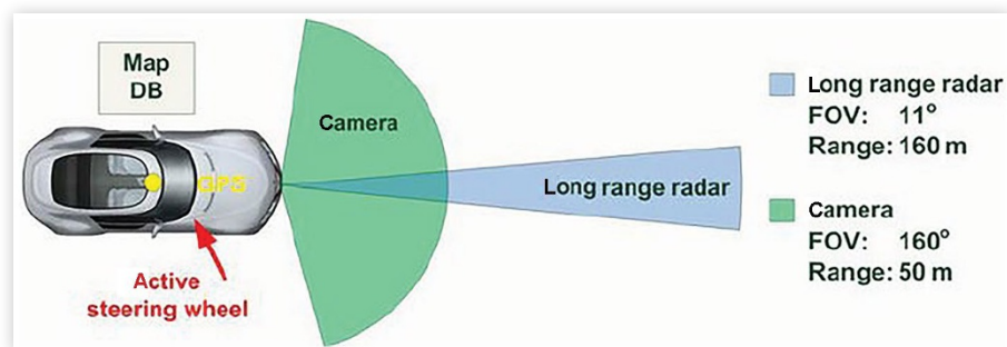
FIGURE 6.16 Sensor fusion application in LKA systems.
