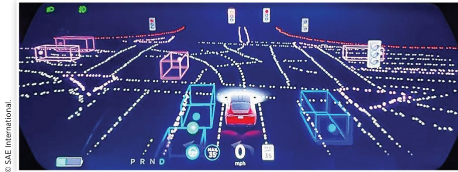
FIGURE 5.23 A screenshot of the perception results of a Tesla Model 3 with FSD on the dashboard of the vehicle.
