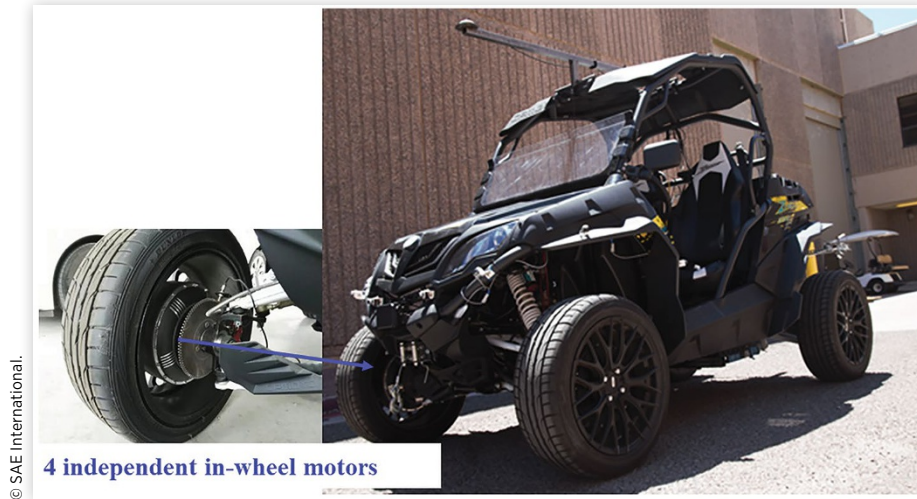
FIGURE 4.23 A CAV driven by four independent in-wheel motors.
