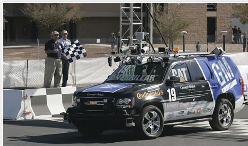
FIGURE 7.6 CMU’s winning entry to the 2007 DARPA Urban Challenge, “Boss,” employed a finite-state machine driving logic.
