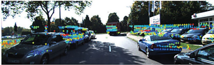
(c) Ground plane removal and projection of laser points on vertical surfaces
