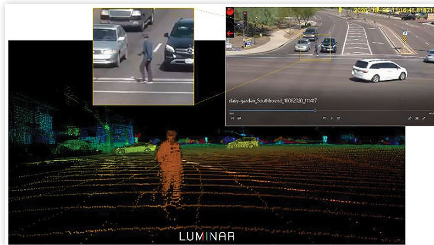
FIGURE 9.10 Sample LIDAR data collected from Anthem testbed with corresponding traffic camera footage.
