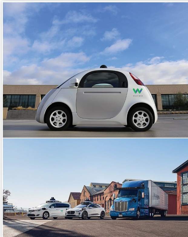
FIGURE 9.1 Early Waymo autonomous driving technology Firefly (top); Current Waymo fleet (from left) Chrysler Pacifica PHEV and Jaguar I-Pace for Waymo One robo-taxi service and the Class 8 long-haul truck for Waymo Via (bottom).
