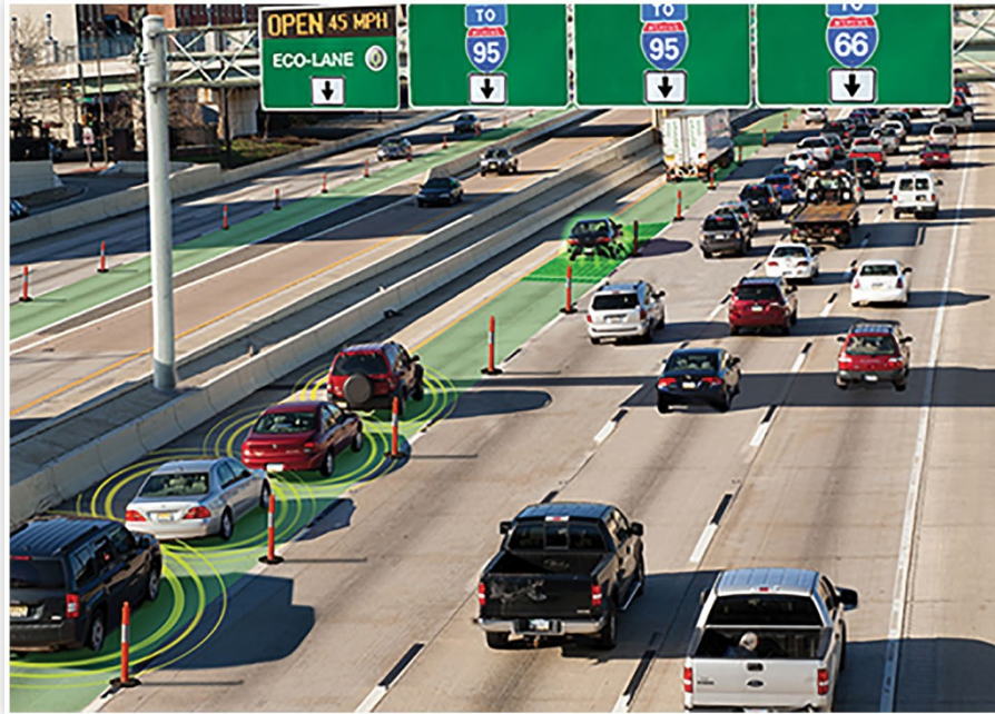
FIGURE 3.5 Platooning of connected vehicles in an “eco-lane.”
