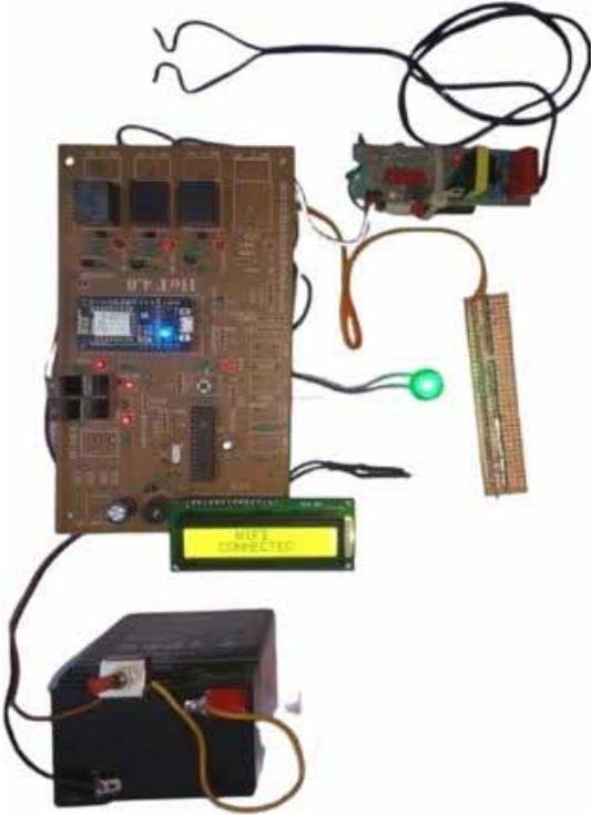
Figure 4. Hardware Module while WiFi connected
