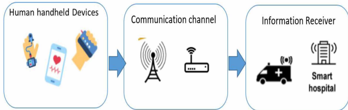
Figure 2. The edge devices (or) sensor connected to the Internet of Things (IoT) health care system
