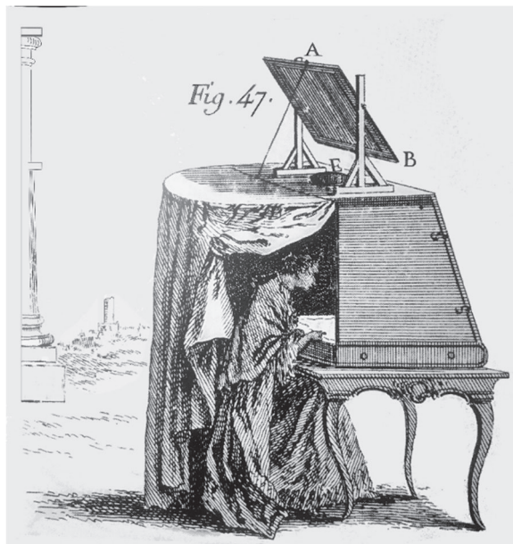
Fig. 3.4 - Porta’s application of the improved camera oscura : AB is a mirror inclined at 45^\circ to the horizon; E is a convergent lens that projects the image of an external object on to a sheet of drawing paper. Source: A. Saverien, Dictionnaire universel de mathématique et de physique , Paris 1754.
