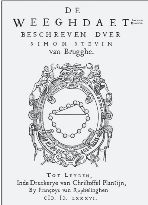
Fig. 3.3 - Frontispiece of Stevin's pamphlet on statics with a drawing of a rosary wrapped on two inclined planes (Leyden 1586).
