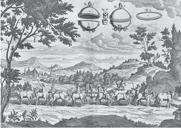
Fig. 5.8 - The experiment of the “hemispheres of Magdeburg”. Illustration from Guericke’s Experimenta .
