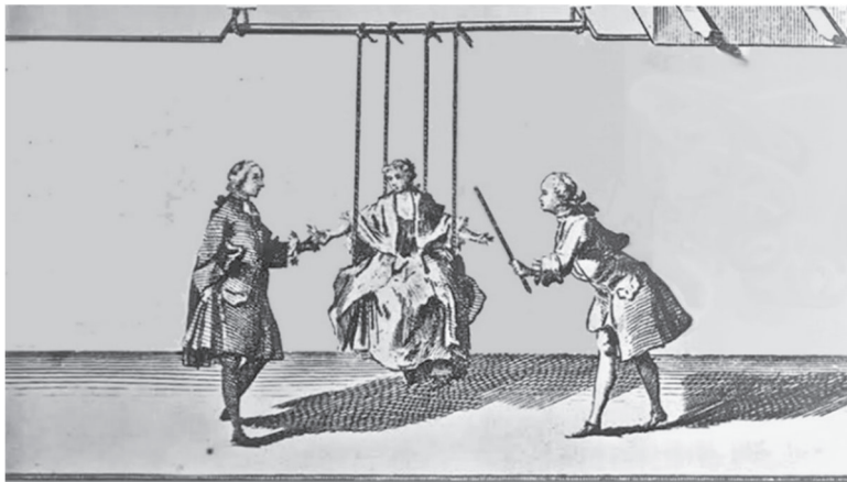
Figure 7.7 - Gray's experiment, from a 1754 incision; the person on the right brings an electrified glass tube close to the woman suspended by silk ropes and the man on the left is struck by a spark.
