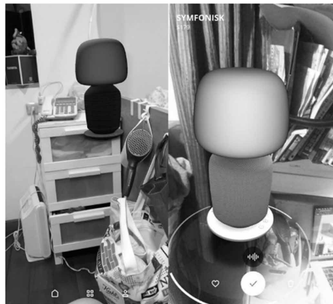
Figure 6. Virtual objects placed in the wrong position due to flawed plane detection (screenshot by the participants)
