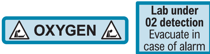
Fig. 11.2: Alarm warning and door panel indication.
