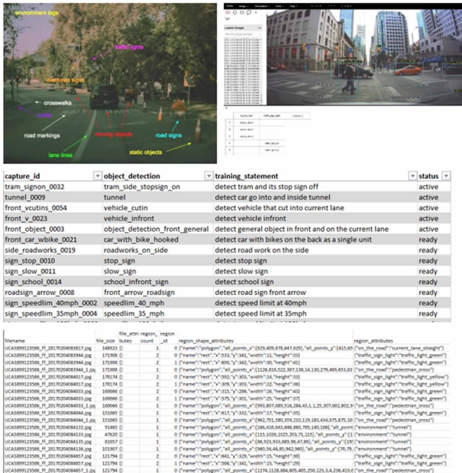
Figure 8. Using a highly simplified demonstration, images sent from the fleet need to be preprocessed, one of the most important steps is to annotate all the important environmental tag, especially those that are novel and never or rarely seen by the neural network. Those annotation can be store in multiple format, including CSV and JSON and will be fed together into the training with the related images. (credit image on top left: Karpathy, 2019)
