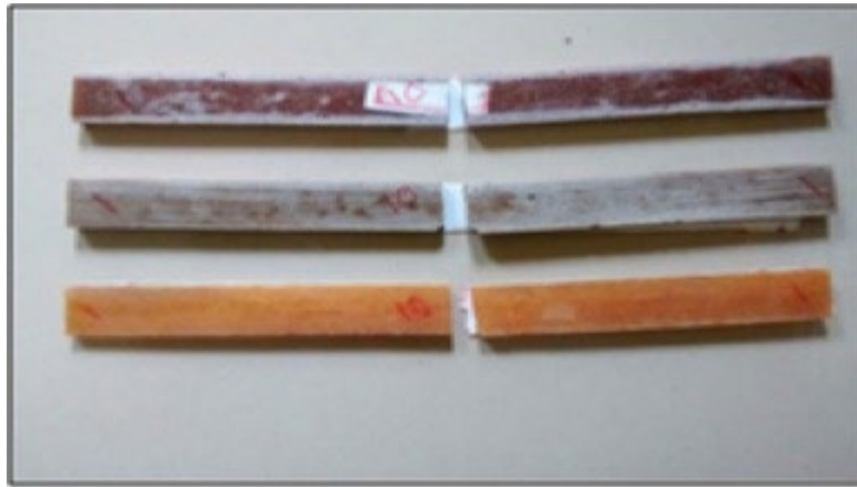
Figure 10. EP, EO and EC specimens failed under flexural load
