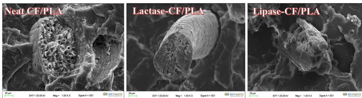
Figure 3. SEM micrographs of neat and enzyme-treated coconut fiber containing PLA composites.
