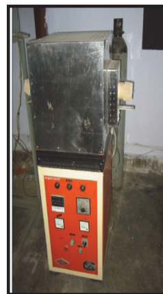
Figure 2.6: PID controlled furnace.
