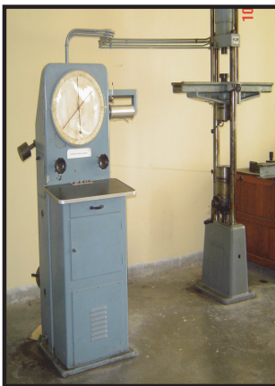
Figure 2.5: Powder compaction press.
