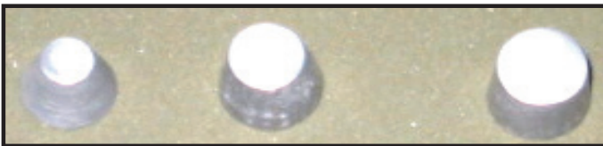
Figure 2.7: Truncated conical Aluminium metal powder preforms.
