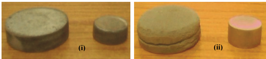
Figure 2.9b: Copper metal powder preforms after forging under (i) lubricated conditions; (ii). dry conditions
