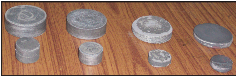
Figure 2.9 (a): Aluminium metal powder compacts with varying l/d ratio.
