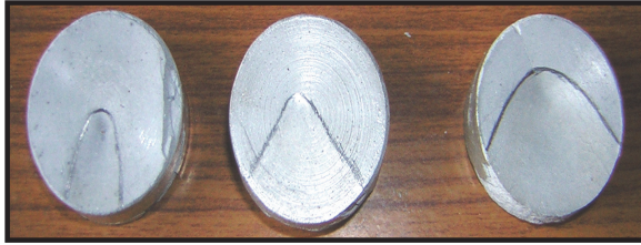
Figure 2.29 (a): Indented area after indentation phase of rotary sinter-forging.
