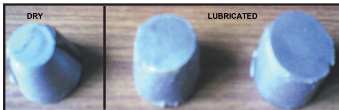
Figure 2.24: Aluminium metal powder truncated conical preforms sinter-forged under dry & lubricated interfacial friction conditions.
