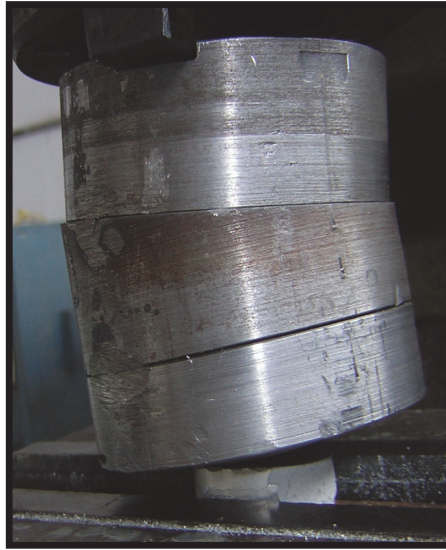
Figure 2.27: Rotary sinter-forging of powder preform.
