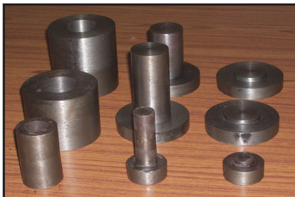
Figure 2.1 (c): Powder compaction die sets with varying diameters.
