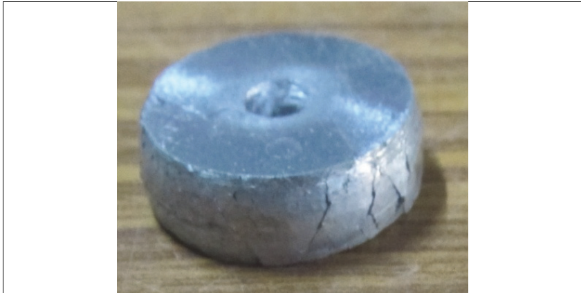
Figure 3.23: Formation of Cracks on Hollow Disc Preform.
