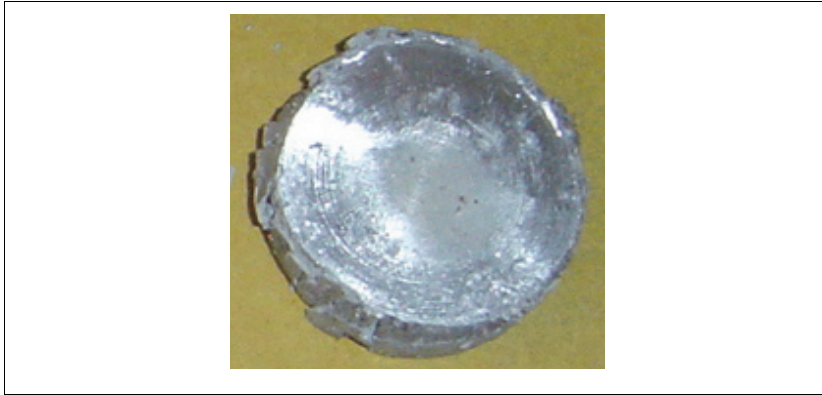
Figure 3.14: Formation of Cracks on Cylindrical Aluminium Preform.
