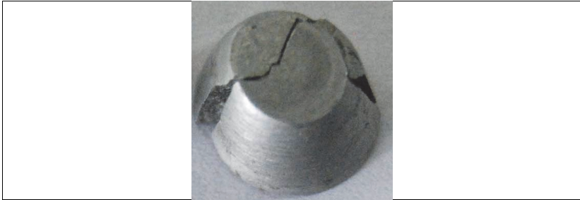
Figure 3.27: Formation of Cracks on Truncated Conical Preform.
