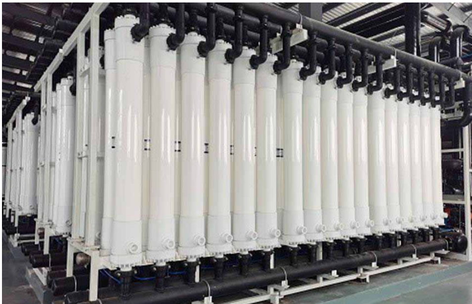
Figure 4. Membrane developed by Toray Company that might be used in lithium extraction
