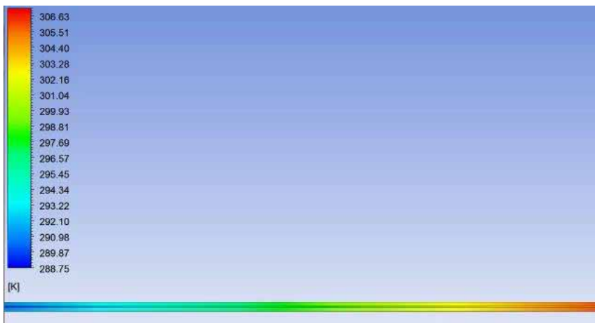
Figure 12. An example of a profile of the temperature along the regenerator
