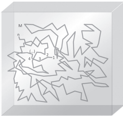
Figure 7.16 The M-molecule moves in an infinite environment due to Brownian motion caused by the heat in the molecule itself and by collisions with solute molecules.
