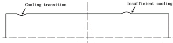
Figure 1. Emulsion cooling causes local crown changes of rolls
