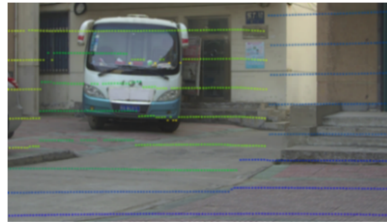
Figure 4. Joint calibration of camera and lidar
