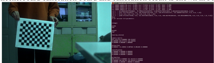
Figure 3. Calibration of monocular camera
