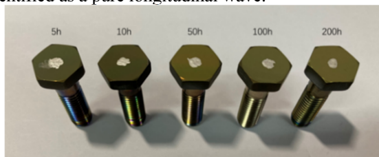
Figure 5. Bolt samples after different annealing time at 300 °C.
