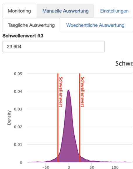
Figure 1. Density plot of relative changes of the median (y) for ft3 values with corresponding thresholds (Schwellenwert), for which only the right one (here the 90% percentile) is relevant in our datasets.
