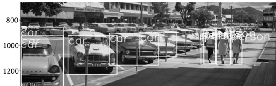
Figure 16.6: Applying YOLOv3 on an image of a street with cars
