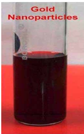
Figure 2. Chemically prepared gold nanoparticles (AuNPs) suspended in liquid
