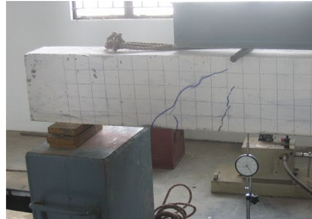
Fig. 6 Shear crack on Reinforced Concrete with minimum stirrups beam
