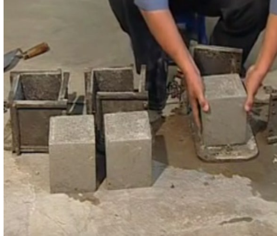
Fig 11: Demoulding of cubes
