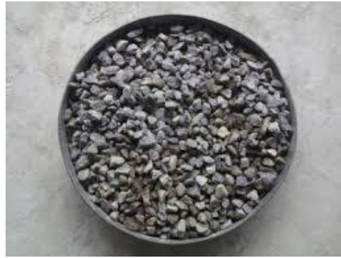
Fig 3: 20mm coarse aggregate
