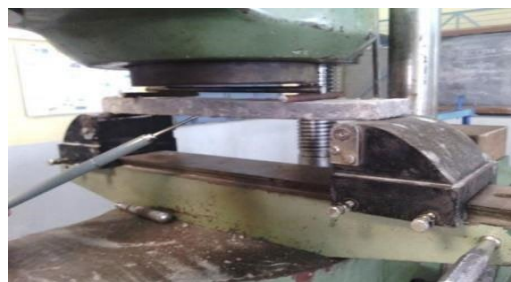
Fig. 3 Photographic View of Slab Testing on Universal Testing Machine
