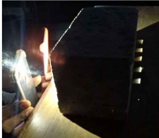
Figure 7 (a) Light emitting property of translucent block
