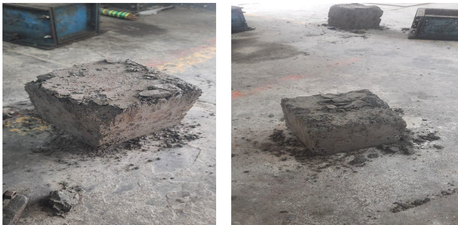
Fig 14: Failure while de-moulding
