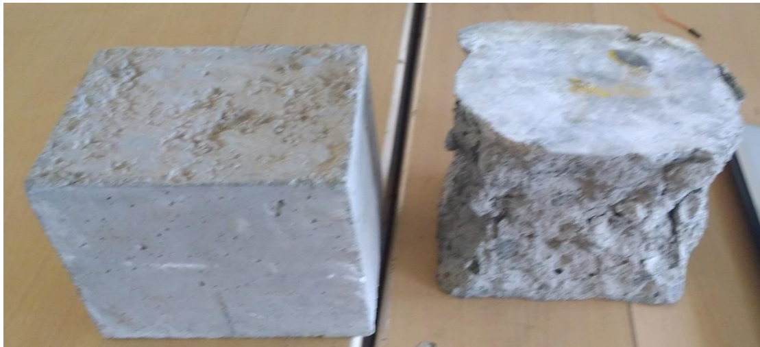
Fig. 8. Concrete specimens (a) before damage and (b) after damage
