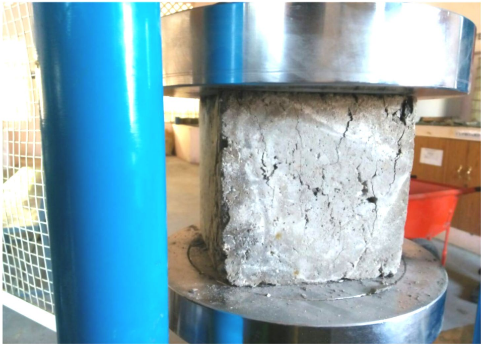
Fig. 2: Compressive Test of Concrete Cube
