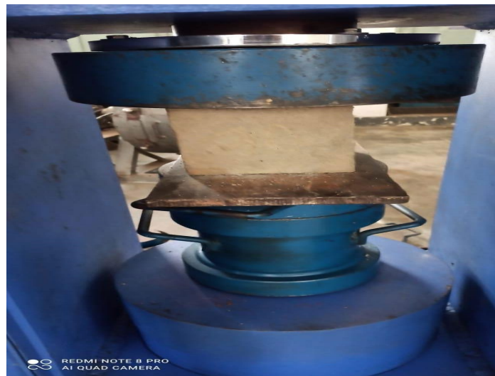
Fig 12: compression testing using UTM
