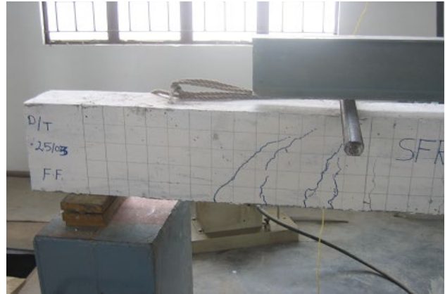
Fig. 8 Shear Crack on SFRC Beam
