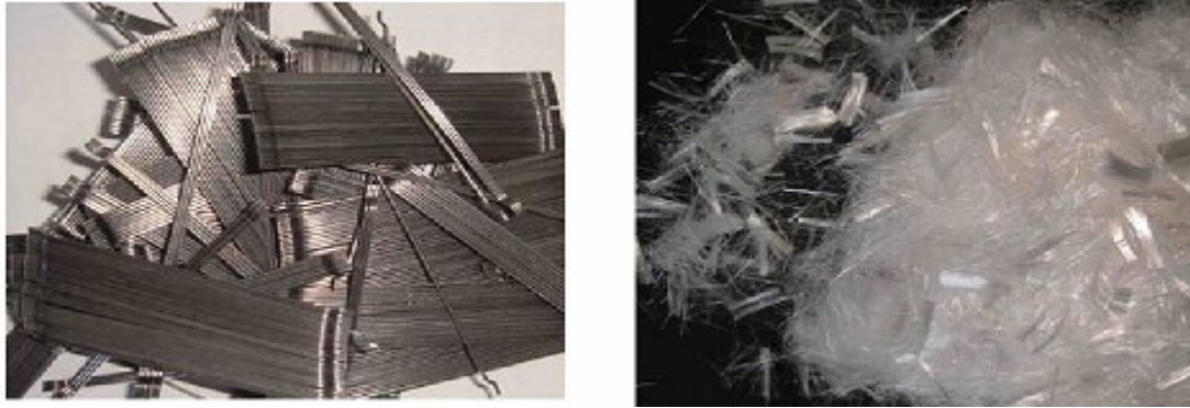
Fig. 1 Glued DRAMIX Steel Fiber and Polypropylene Fiber
