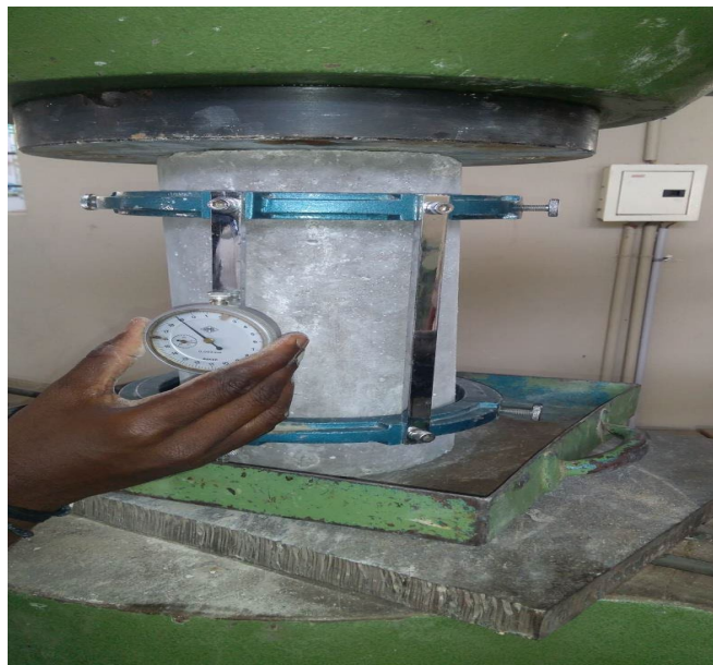
Fig.8 – Modulus of elasticity test set up
