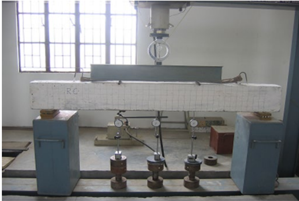
Fig. 3 Experimental set-up of beam with loading frame in laboratory
