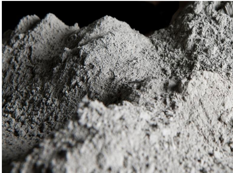
Figure.1 Ordinary Portland cement
