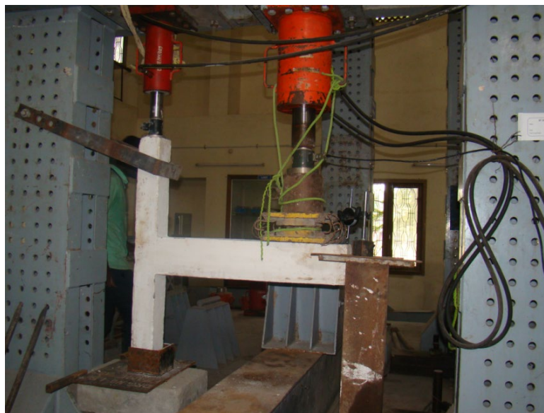
Fig. 2. Test set up of exterior joint of beam-column
