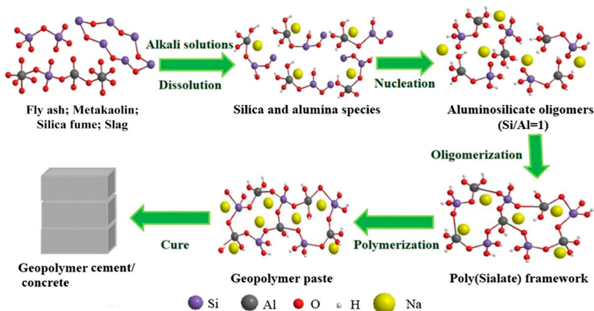
Fig. 1. Geo polymerisation Process [2,3]
