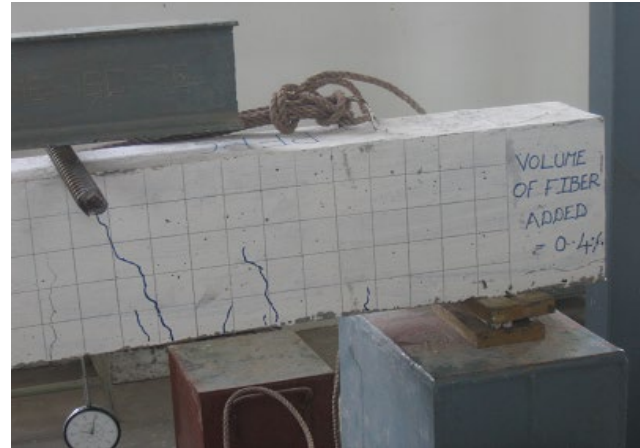
Fig. 10 Shear Crack on PFRC Beam
