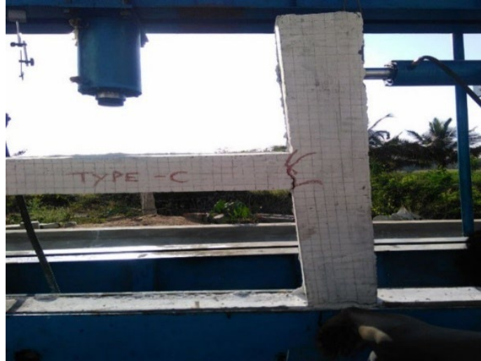
Fig.3. C type reinforcement loading
