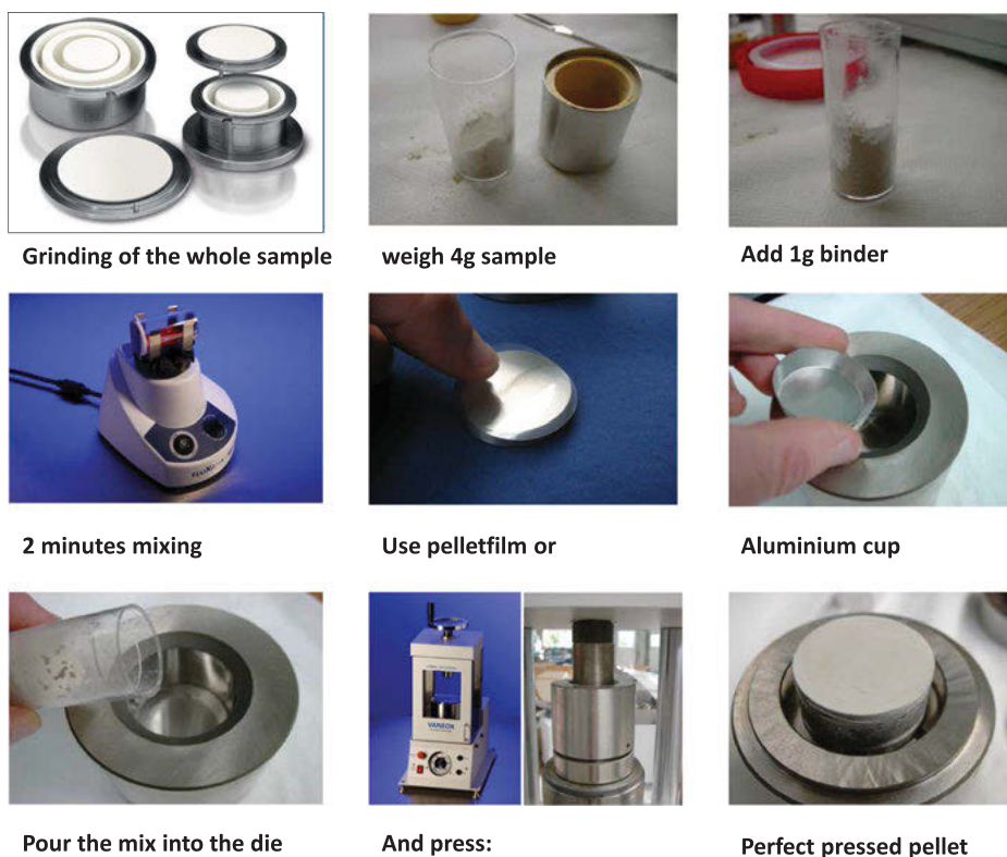
Figure 9.7: Illustration of all steps to produce a pressed pellet with binder.
