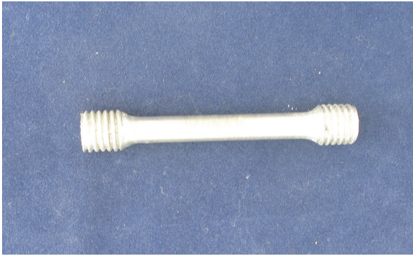
Figure II-2-8 A photograph of a typical form of a test piece (test specimen) used in the mechanical testing of metals/alloys (provided by R. Lazarova).
