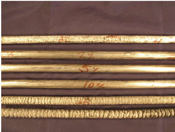
Figure I-3-1. Extruded bars with w = 0, 2, 5, 10, 15 and 20 wt. % TiCN
