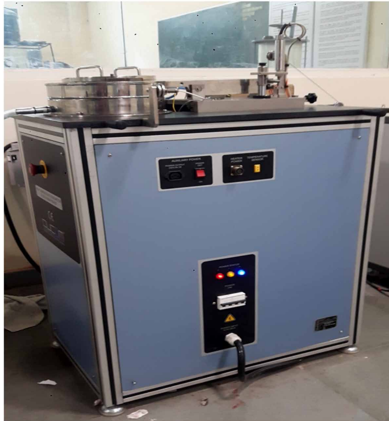
Figure 3. Camera picture of high temperature pin-on-disc tribometer
