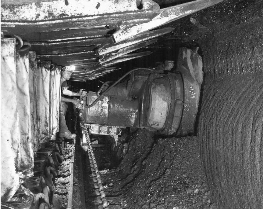
Figure 4.11 Shearer on 93's face (Thoresby) in 1976 (photo credit: Coal Authority)
