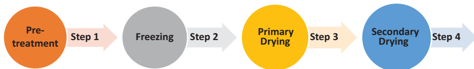
Figure 12.10: The four basic steps of the freeze-drying process.
