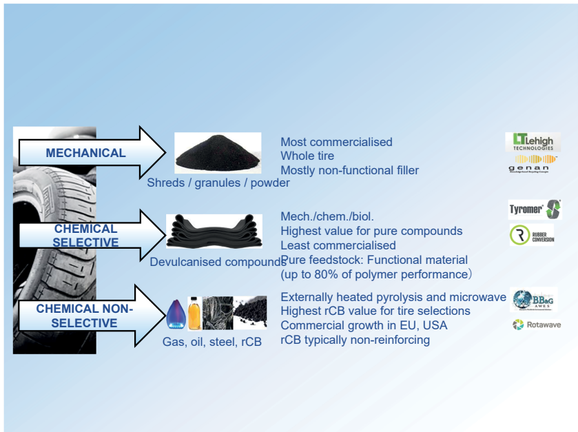
Figure 9.3: Tire recycling processes.
