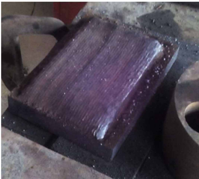
Figure 18. WAAM sample deposited by KUKA robot.
