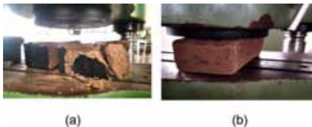
Figure 3. Compression Strength using UTM for (a) painted brick and (b) unpainted burnt bricks
