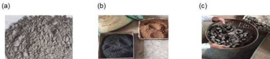
Figure 3. (a) Cement; (b) Fine aggregates river sand and M-Sand; (c) Coarse aggregates
