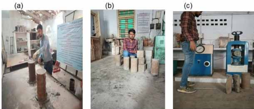
Figure 6. (a) Molded cylinders; (b) Specimens; (c) Cracks developed in cylinders in Split Tensile testing
