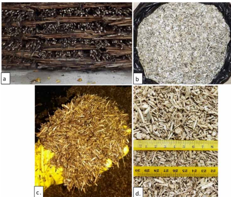
Figure 1. Sunflower stalks aggregates obtaining: a. drying of sunflower stalks; b. appearance of sunflower stalks after shredding; c. appearance of crushed sunflower stalks treated with sodium silicate solution, in the wet state; d. appearance of sunflower stalks after treatment with SS, in dry state
