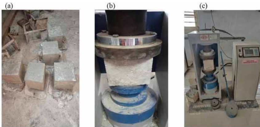
Figure 5. (a) Moulded cubes; (b) Testing on cubes; (c) Cracks developed in cube during compressive testing
