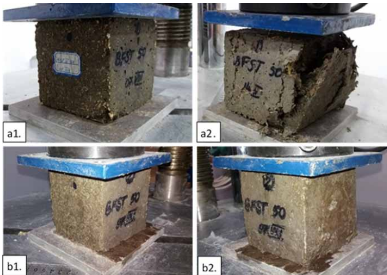
Figure 10. Freeze-thaw resistance test: a. vegetal concrete specimen subjected to freeze-thaw cycles, before (a1) and after (a2) compressive strength testing; b. vegetal concrete control specimen, before (b1) and after (b2) compressive strength testing
