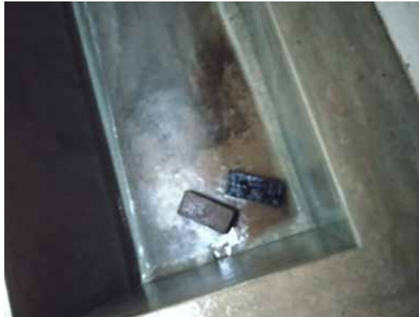
Figure 4. Water absorption test
