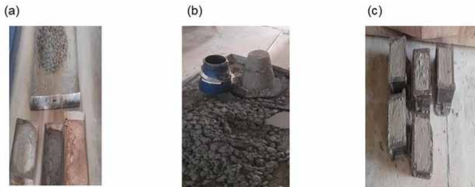
Figure 4. (a) Materials; (b) Slump Cone Test; (c) Moulds filled with concrete
