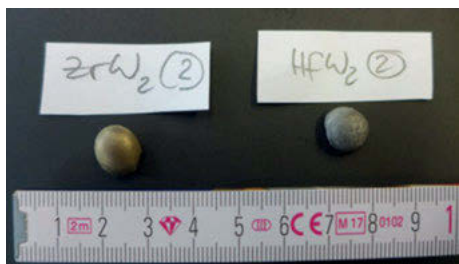
Fig. 13.25: Two samples of approximately 5 g of ZrW 2 and HfW 2 . ZrW 2 has a more “golden” color, whereas HfW 2 is silvery-metallic.
