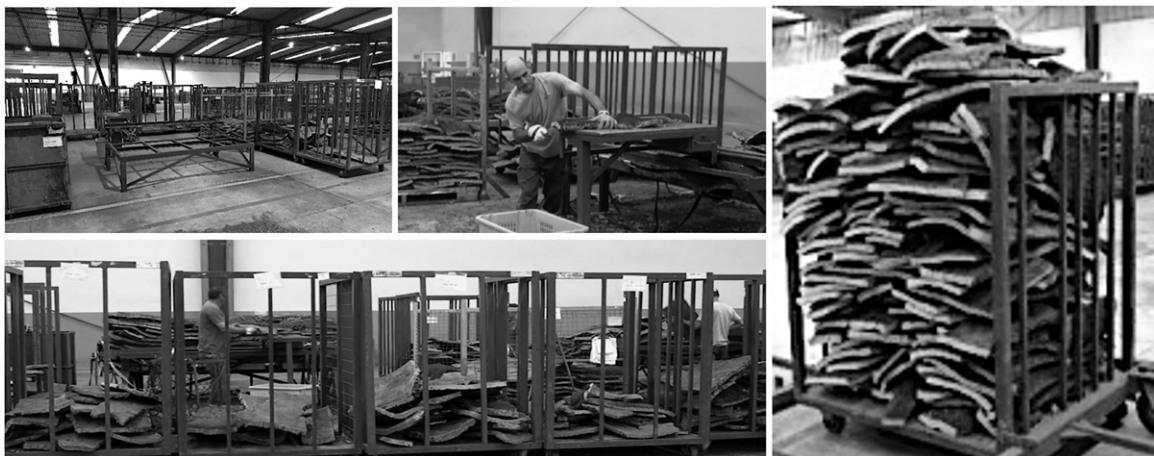
Figure 12. Cork sorting bench and cages Source: Industrial cork unit
