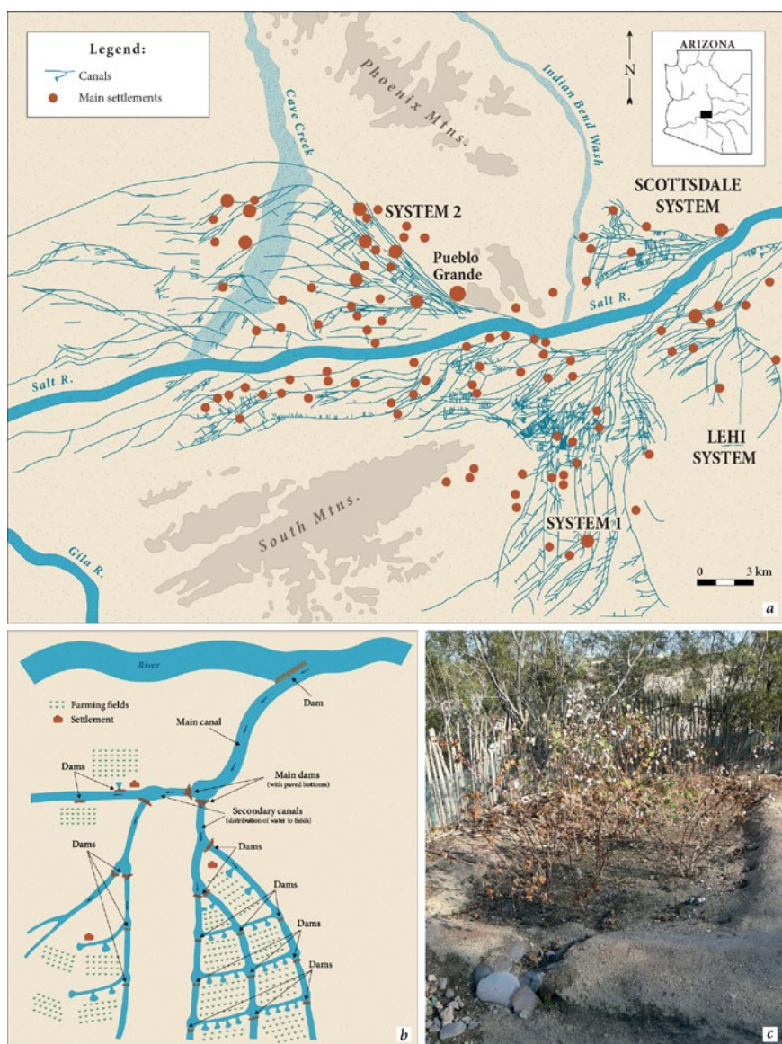
Figure 5.2. The main Hohokam canal systems running from the Salt River (a); (b) reconstruction of water distribution to cultivated plots by a system of first-, second-, and third-rank canals (after Doyel 2007: Figure 10.2 and other sources); and (c) fragments of experimental farming fields with cotton established in situ at the Pueblo Grande. Drawings by Michał Znamirowski (after various sources); photo by Radosław Palonka.
