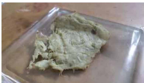
Figure 1. Photograph showing Bio-plastic prepared from raw banana peel
