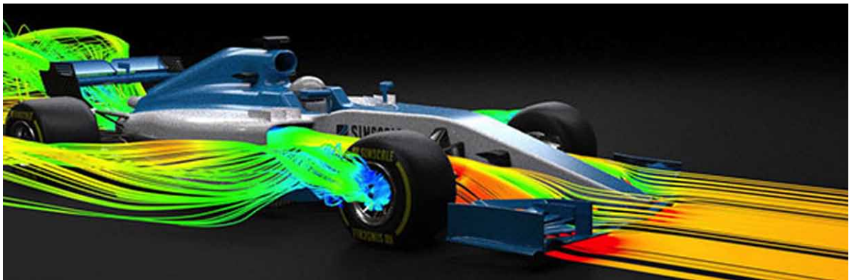
Figure 6. Computational fluid dynamics courtesy to Racecar engineering
