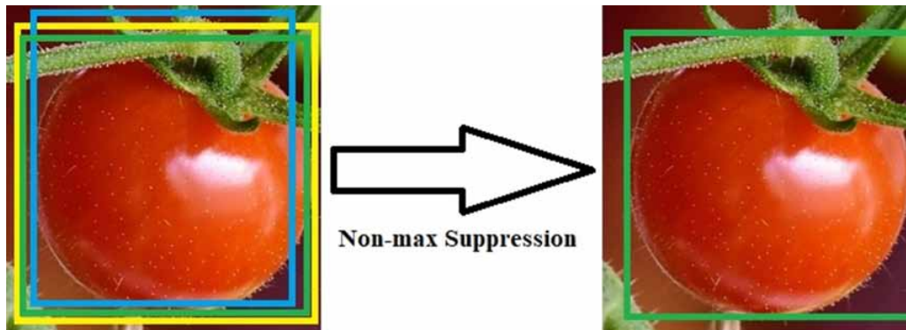
Figure 14. Application of the non-maximum suppression algorithm
