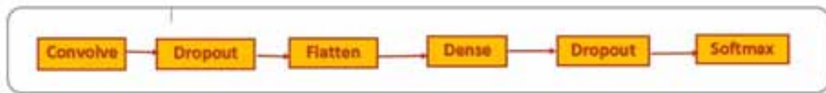
Figure 1. Layers in a convolution neural network (CNN)
