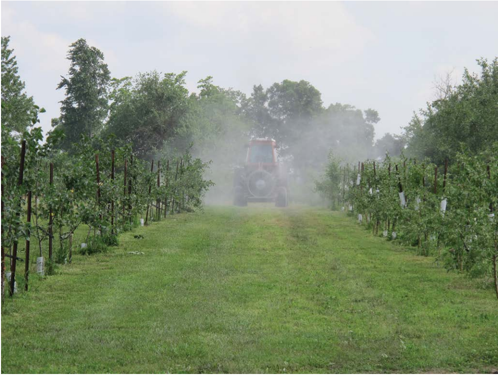
Fig. 9.6. An air blast sprayer engineered with 'smart' technology that uses lasers to turn on and off between trees, reducing the pesticide application. (Authors' own photo.)
