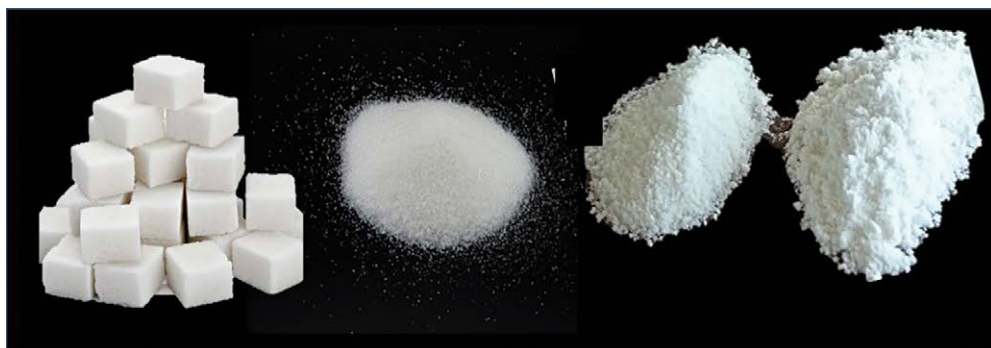
Fig. 7.7. Surface area affects all aspects of pesticide performance and behaviour. For example, a sugar cube (left), 1 cm in size, provides a surface area of 6 cm 2 . Contrast this to sugar, caster sugar or powdered sugar (right) and how the surface area increases by these different millings of sugar. A nanopowder of sugar, 10 nm in particle size, would have a surface area 600 m 2 , sufficient to cover a basketball court and most of the side lines. (Authors' own photo.)
