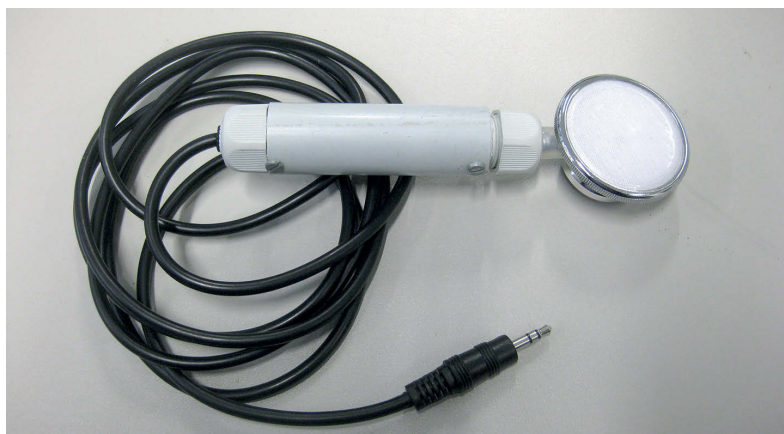
Fig. 4.19: Self-construction of an electronic stethoscope for connection to the PC sound card.
