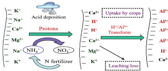
Figure 8.1 Processes of exchangeable \text{Al}^{3+} production during soil acidification (modified from Xu et al. 2018)
