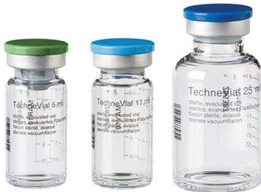
Fig. 12.5: Ready-to-use sterile, evacuated vials (TechneVial™, Mallinckrodt) for elution of the ^{99}\text{Mo}/^{99\text{m}}\text{Tc} generator. Each color of the color-coded vials represents different elution volumes, controlled by different levels of reduced pressure in the vials. Green caps for elution volumes of up to 5 ml; light blue caps for elution volumes of up to 11 ml; and dark blue caps for elution volumes of up to 25 ml.
