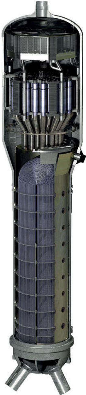
Fig. 10.8: Sketch of a steam generator for an EPR PWR reactor (© AREVA, IMAGE, and PROCESS).
