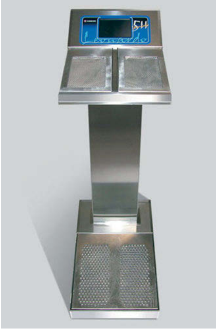
Fig. 1.31: A typical hand-and-foot contamination meter (Comecer S.p.A., Castel Bolognese, Italy). Four plastic scintillators (two for the hands, two for the feet) are read by PMTs and the readout is shown in real-time on the LCD display, after calibration in \text{Bq}/\text{m}^2 for several types of radionuclides (user-selectable). (From http://www.centroditaratura.it/servizi-taratura/strumenti/mani-piedi-vesti/ – last access on June 9, 2012).
