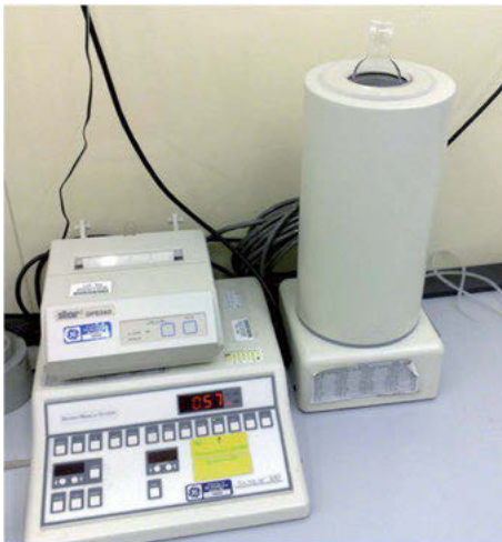
Fig. 1.24: A well-type ionization chamber used for dose calibration in a nuclear medicine department (Biodex Medical Systems, Shirley NY, USA). The ion chamber has an almost 4\pi geometry which maximizes the geometric efficiency. The user can select the type of radionuclide, which allows the correct conversion from exposure (C/kg) to activity (Bq), see eq. (1.28).
