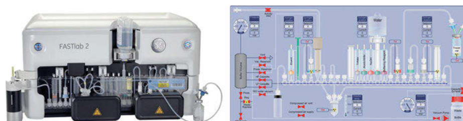
Fig. 12.19: Automated radiosynthesis module (GE healthcare FASTlab2 ® ) for direct nucleophilic ^{18}\text{F} -labeling reactions such as for 2- ^{18}\text{F} FDG, and the corresponding scheme of the Fastlab2-based ^{18}\text{F} FDG radiosynthesis.
