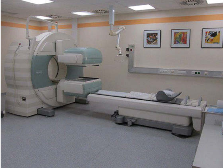
Fig. 12.7: A two-headed SPECT/CT scanner (Siemens Symbia T2) at the Department of Nuclear Medicine of the Hannover Medical School (Germany). The Symbia T2 provides two rotating gamma detector units (“heads”) for SPECT and a two lined CT system.
