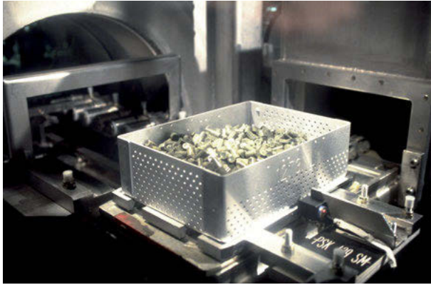
Fig. 10.19: Raw pellets before entering sintering furnace, Melox MOX fuel fabrication plant, Bagnols-sur-Cèze, France (© AREVA, Patrick Lefevre).
