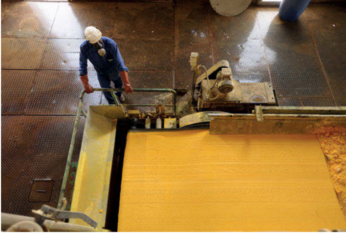
Fig. 10.16: Somaïr ore processing plant, Arlit, Niger. Yellowcake on band filter (© AREVA, Jean-Marie Taillat).
