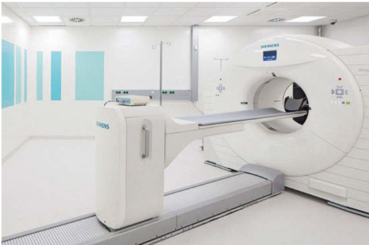
Fig. 12.8: A TOF PET/CT scanner (Siemens Biograph mCT 128 Flow) at the Department of Nuclear Medicine of the Hannover Medical School (Germany). The Biograph mCT 128 Flow consists of a 128 lined CT and a PET including TOF registration. The 128 lined CT allows full body CT scans within only a few minutes. The flow technology enables scans with continuous moving of the patient/bed instead of stepwise protocols.
