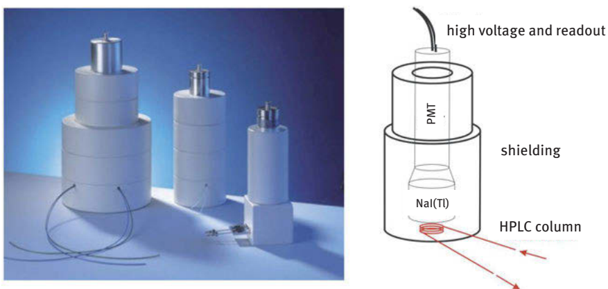
Fig. 1.27: Example of gamma radiation detector for radio-HPLC (raytest Isotopenmessgeräte GmbH, Straubenhardt, Germany). A thick lead shield protects the scintillator detector against undesired events from the background activity. The HPLC column passes through two small holes in the shield walls at the base of the apparatus. A small loop in the column provides a local increase of the measured activity (and hence an increased sensitivity) nearly at contact with the detector window, leading to an almost 2\pi geometry. (Photograph from www.raytest.de , last access on June 9, 2012).
