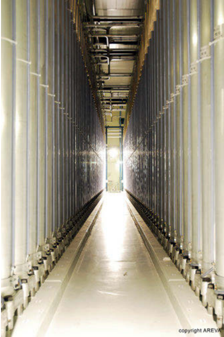
Fig. 10.18: Rotation of first centrifuge cascade. George Besse II site unit 1. December 9, 2009 (© AREVA, Nicolas Petitot).
