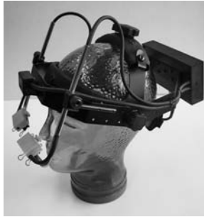
(b) Head-Mounted Eye Tracker: SMI's EyeLink II
