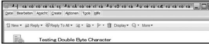
Figure 1. An example of poor internationalization. In this instance a process for rendering window titles did not know how to properly interpret text not in the Roman script and “garbled” it. (Example courtesy of Dale Schultz, IBM.).
