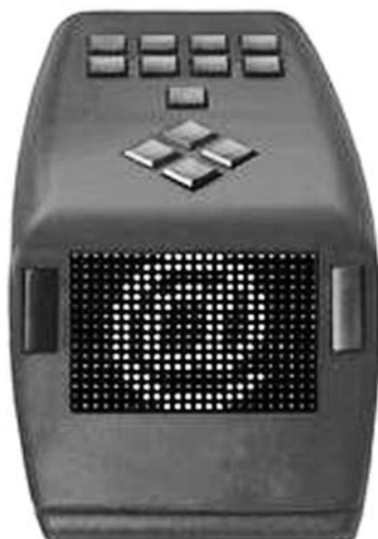
Figure 4. The electronic pin display Graphic Window Professional (GWP) displaying the “@” sign (figure taken from https://www.handytech.de/index.php?id=26&L=0 , accessed June 1, 2011).
