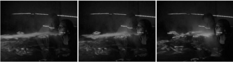
Fig. 5-2. Laser-light and fog used to observe a woman's breath as it travels over six metres through the warehouse space.
