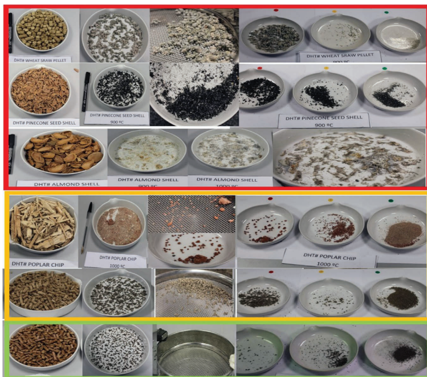
Figure 3: SaG method results from the Domoheat Project. Severe slagging was measured for rye straw, pinecone seed shell and almond shell fuels, with high amounts of calcinated weight and high percentage of melted and sintered fuel. The right figures show the granulometric distribution ( >2 , >1 and <1 mm) of the calcinated samples. Unlike ash fusion or rapid tests (Fig. 2), medium slagging tendency was measured with the SaG test for soil-contaminated fuels such as poplar chip and pine pellet, corresponding with observed slagging in the boiler combustion tests [18,19].
