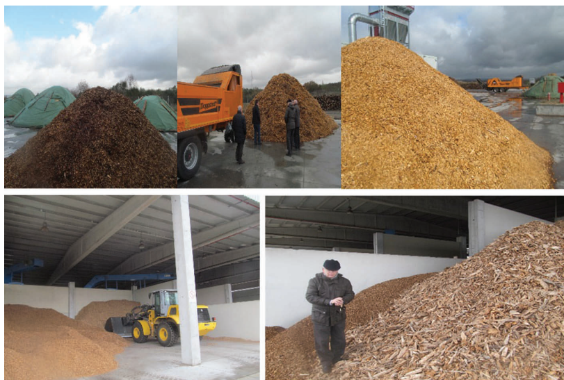
Figure 13: Biomass logistic center in Orense, NW Spain [24]. Woody biomass is chipped after storage and dried under open air conditions. Chipped wood and bark are screened for the production of wood chips of normalized sizes P16–P90.
