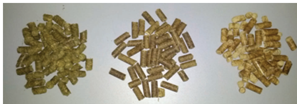
Figure 1: Pellets made from different types of residual biomass under different pelletization conditions.
