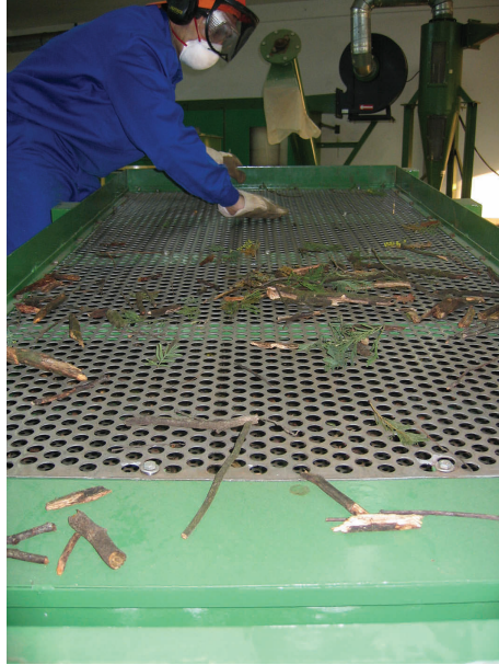
Figure 11: Screening of residual forest biomass at the Forest biomass pilot plant of the Faculty of Forest Engineering, University of Vigo [18].
