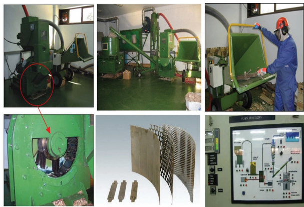
Figure 10: Details of the forest biomass densification pilot plant of the Faculty of Forest Engineering, University of Vigo, with a detail of the patented milling hammer system [22]. More information of the pilot plant can be found at: http://ortiz.webs.uvigo.es/?page_id=20
