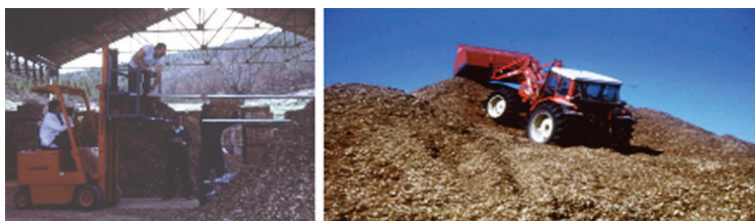
Figure 3: Open air natural drying of wood chips at the CIEMAT Renewable Energy Centre in Soria, central Spain [17,18].
