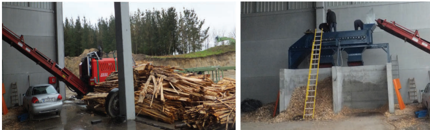
Figure 12: Biomass logistic centre in Palas de Reis, NW Spain [24]. Top figure: woody biomass chipper and debarker. Bottom figure: a screen with variable opening size is utilized for controlling the granulometric distribution of wood chips to a P31 or P45 size category. Fine fractions of <8 or 16 mm are separated for pellet production.
