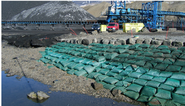
Figure 2: Testing the use of geobags to reduce erosion at Svea mine, Spitzbergen (Caline [7]).
